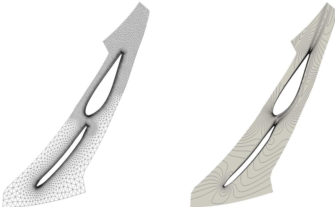
Figure 6.21: Mesh generated by H2OMESH with a structured layer and isocontours of the velocity field computed by CFX.
