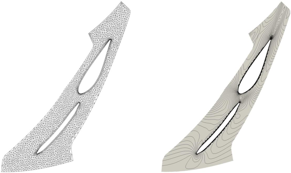
Figure 6.22: Generic Delaunay mesh generated by `TriDelta` and isocontours of the velocity field computed by CFX.
